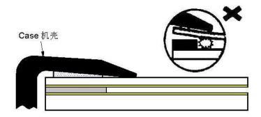
9) Wipe off the stain on the product by using soft cloth moistened with ethanol. Take care not to allow ethanol to soak into the joint of upper Film and bottom glass. It may otherwise cause peeling or defective operation.
