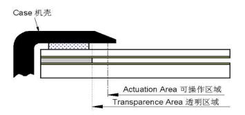
6) a. Pressing inside of boundary of the frame(part (A) as shown in below) may causes fault operation, so please design to avoid pressing of touch panel at part (A) such as having gasket/cushion at part (C). Particularly the area (B) shall be free from burr. The gasket/cushion material at the part (C) should not be exceeded to inside of the boundary of the frame.
