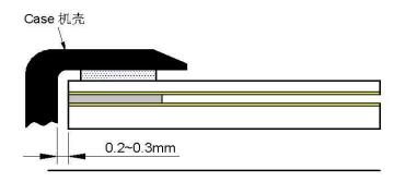
Meanwhile, in order to avoid touch panel any failure for extra wrap tail, please take care of keeping clearance of 2.0min.between tail position and inside boundary of case when the touch panel is built into case.
