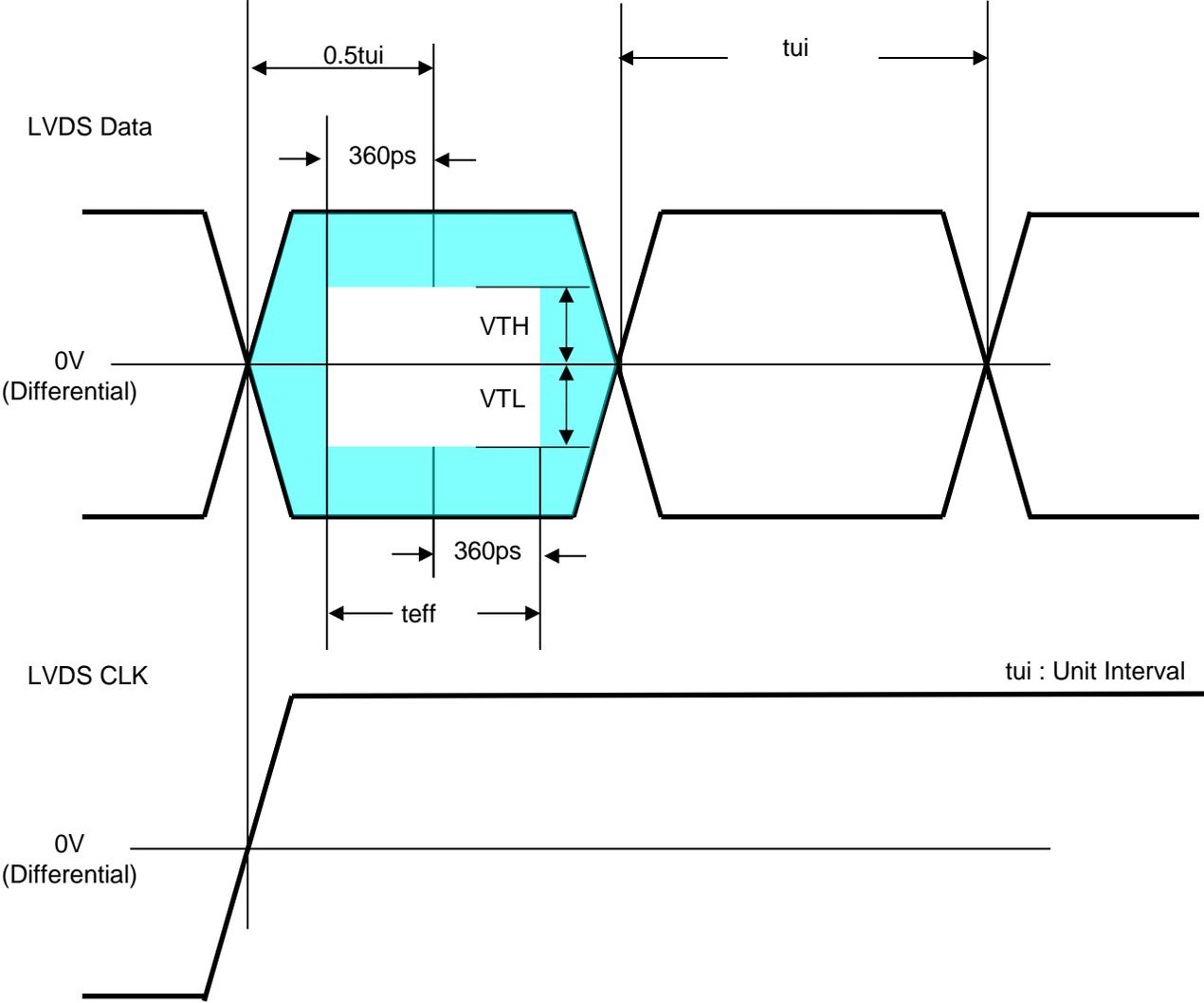
\* This accumulated waveform is tested with differential probe
