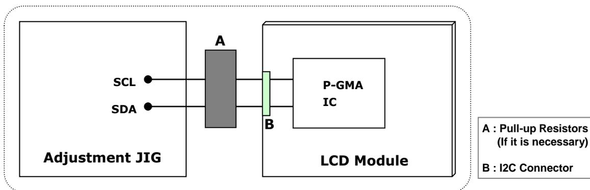
FIG. 8 VCOM Adjustment Pattern & Block Diagram
