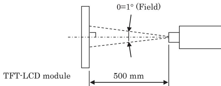
The luminance is measured according to FLAT PANEL DISPLAY MEASUREMENTS STANDARD (VESA Standard).
