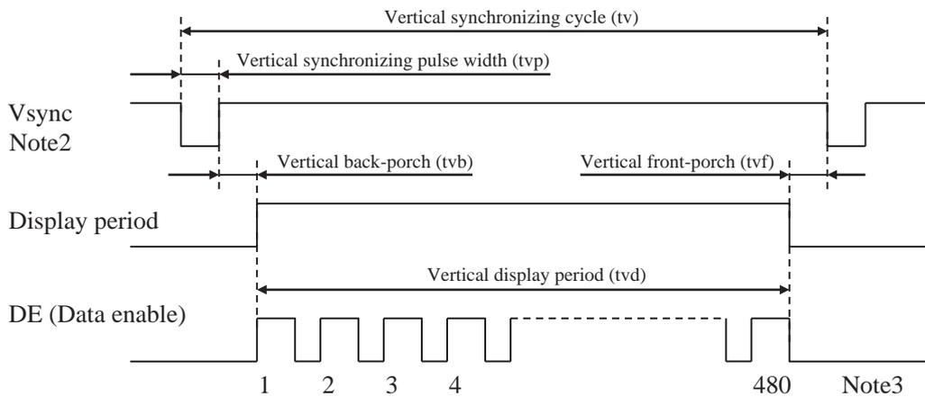
Note1: This diagram indicates virtual signal for set up to timing.
