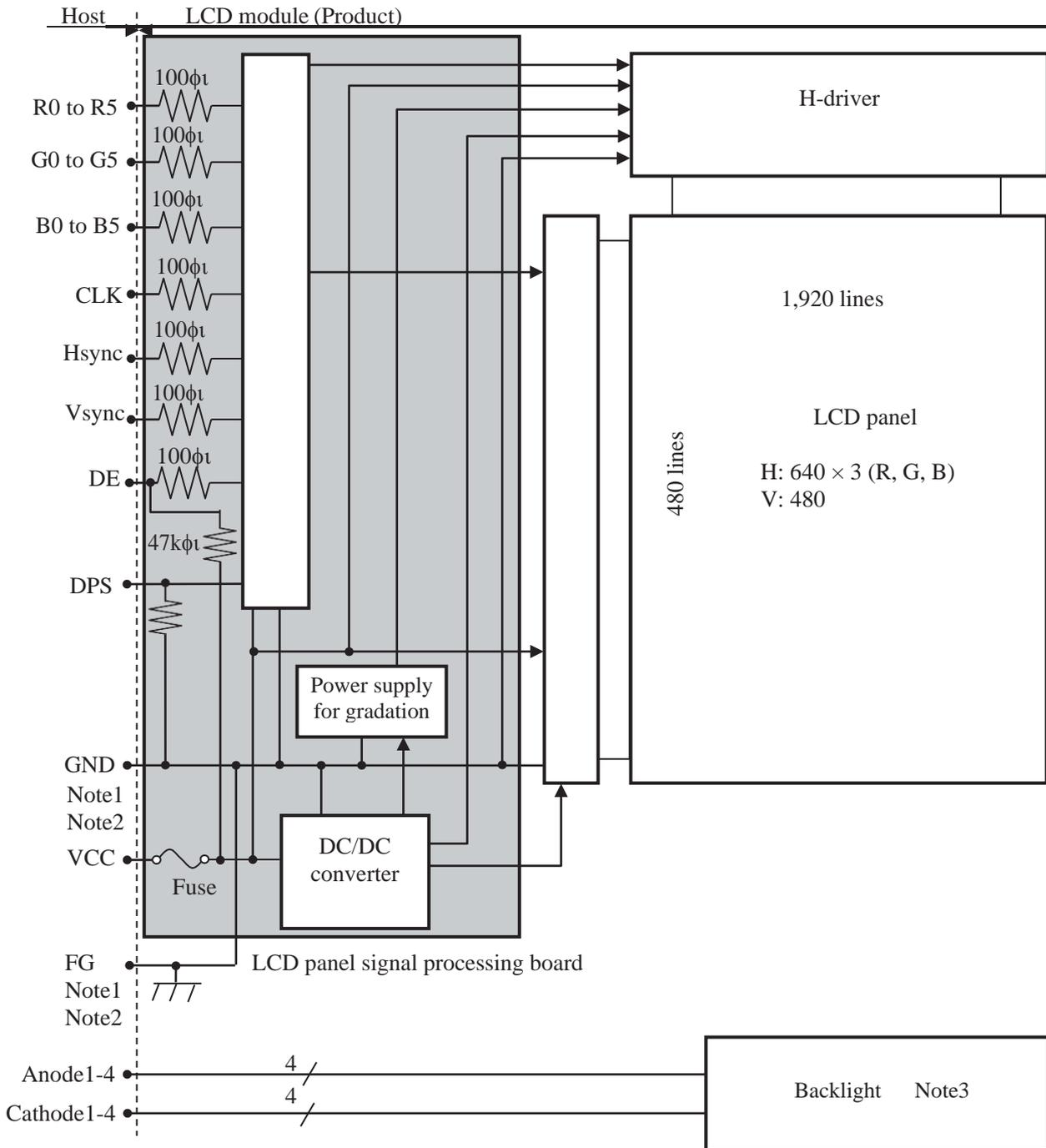
Note1: Relations between GND (Signal ground) and FG (Frame ground) in the LCD module is as follows.
