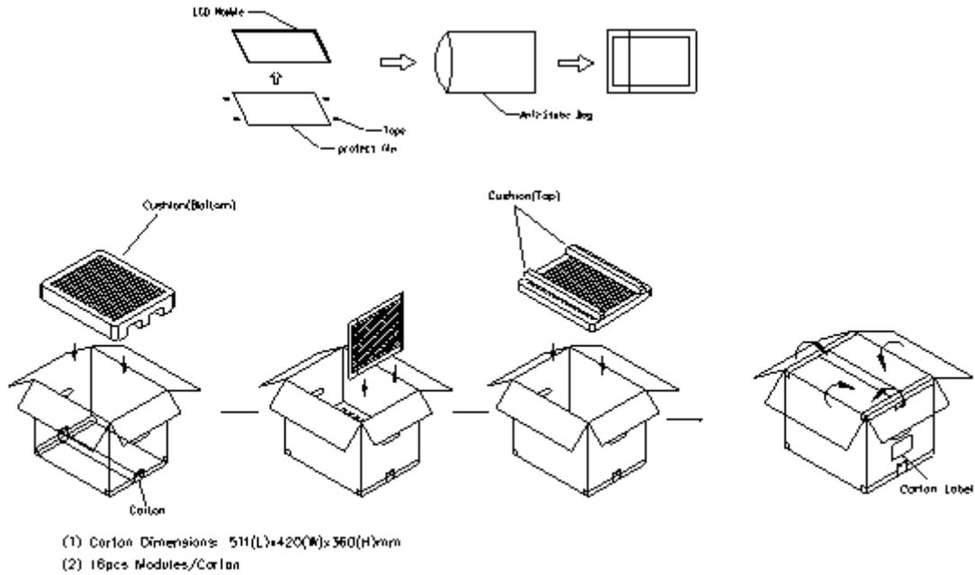
**Figure. 9-1 Packing method**
