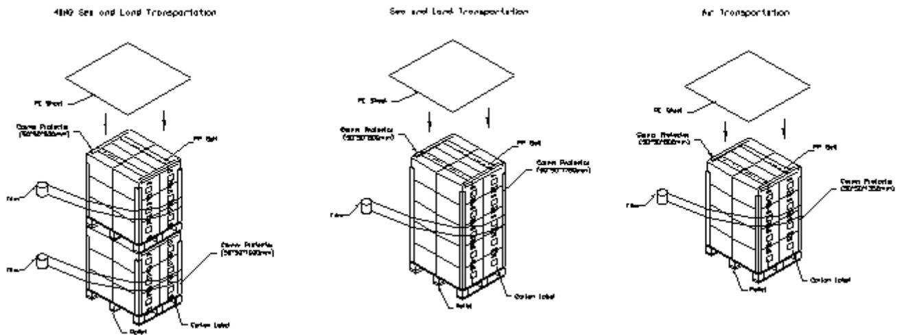
**Figure. 9-2 Packing method**
