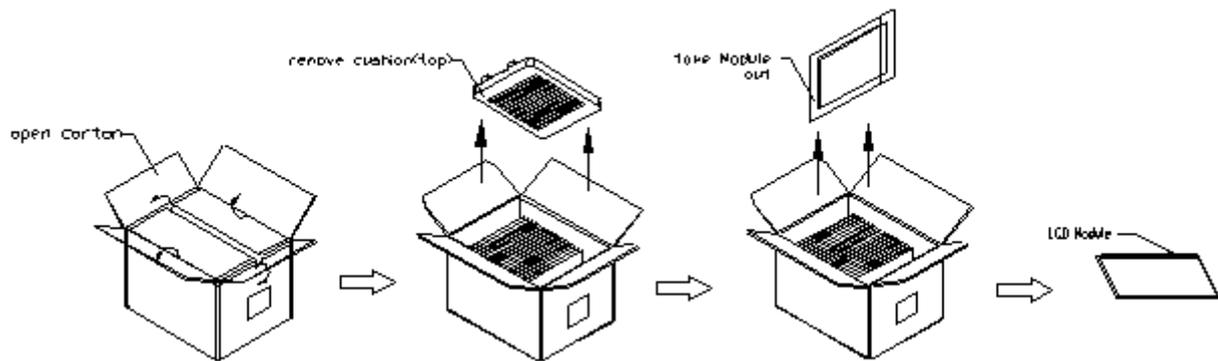
Figure. 9-3 UN-Packing method
